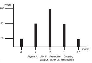
to note that there is no increase in output power below the 2 Ohm threshold. Maximum power is achieved at 2 Ohms. AM III provides you the satisfaction of knowing that your ArtSeries amplifier will continue to play when momentary impedance dips occur. (Refer to figure A)
