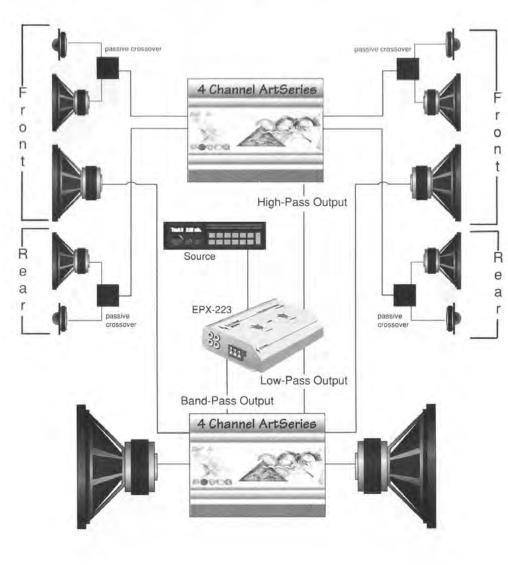
Bi-amp System utilizing EPX-223 crossover band-pass output for front mid-bass drivers
