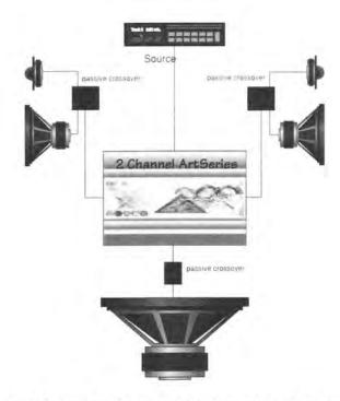
Mixed Mono System utilizing passive crossovers: Two Channels Stereo with derived Mono Channel
