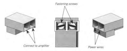
Figure C Power / Ground Connector
