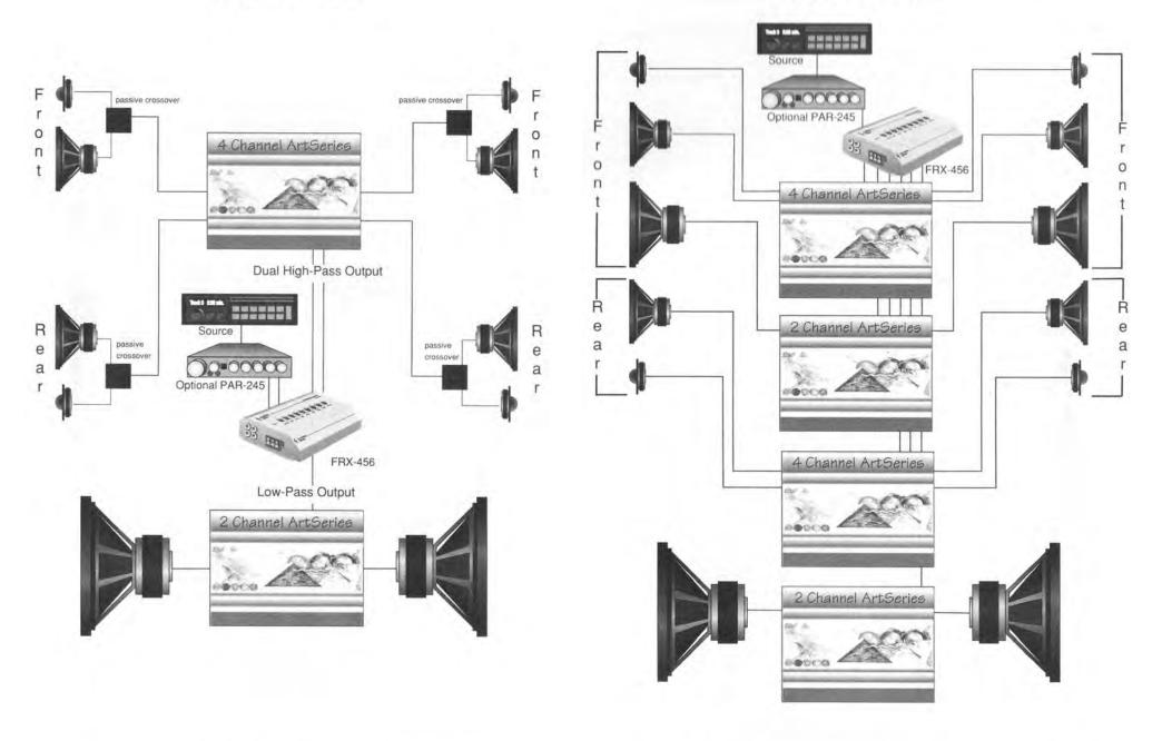
Bi-amp System utilizing FRX-456 crossover with front/rear fade capability
