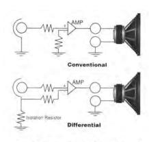
Figure B. Conventional vs Differential Inputs
