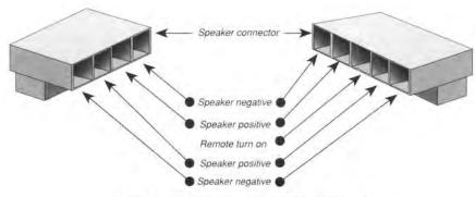
Figure D. Speaker / Remote Turn-On Connector
